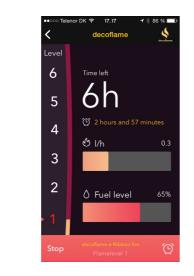
6. For adjusting the flame intensity, select the desired numeric level displayed on the left side of the screen (1-the lowest intensity; 6- the highest intensity).
