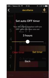
5. The power off timer can be activated by selecting the timer icon situated in the lower right corner. To choose the remaining burning time, slide the dot on the bar accordingly and then select "SET TIMER". The countdown timer will be visible also when returning to the main App page. The remaining burning time can be changed by following the above mentioned steps. To cancel the timer, select "CLEAR TIMER".
