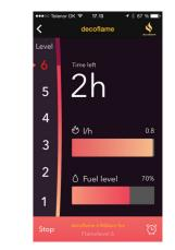
4. When you access the decoflame<sup>®</sup> App, it is possible to start the fireplace by selecting the "START" icon. If the fireplace has already been turned on using the display, you can now monitor the fuel level and calculate the fuel consumption.
